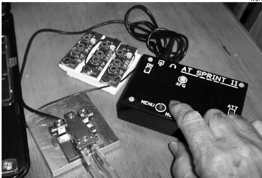
**Figure 4 — The AT Sprint II covers 80, 40, 30 and 20 meters. It has a direct digital synthesizer VFO and covers a 150 kHz range. The superheterodyne, single-conversion receiver has a 4.9512 MHz IF. The FET RF power amplifier puts out up to 5 W with 12 V, 2.5 W at 9 V, and 900 mW at 6 V. Output is consistent on all bands.**
